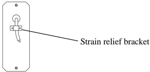
3. You will find a strain relief bracket in the accessory package. Fix the power supply cord below the bracket, as shown in the previous illustration.
