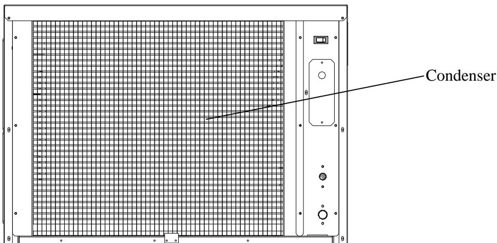
2. The air cooled condenser should be vacuumed once or twice per year to remove any lint that may have been drawn into it. Using a tool that seems like a probe to remove any lint from the condenser fins.
