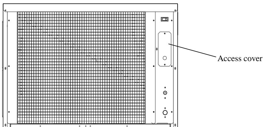
1. Unscrew the two screws holding the access cover and remove the cover. You will find two leads (black and white). See drawing below.
