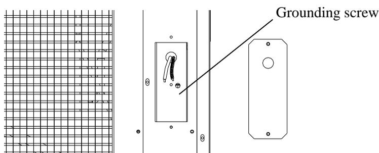
2. Feed a power supply cord (not included) through the access cover and connect it with the two leads. The ground line should be connected to the grounding screw. The two connectors must be insulated. Put the access cover back in place.
