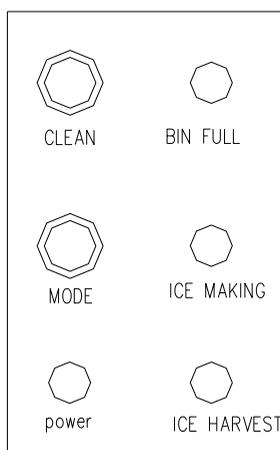
You will find the control panel at the left side of the machine. This panel includes the clean button, the mode button and four LED indicators.
