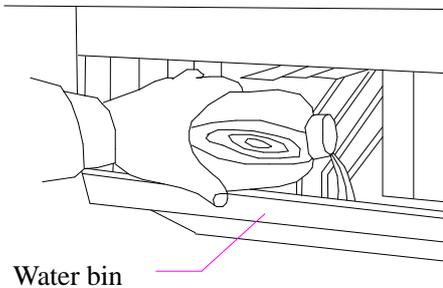
4. Turn on the power to the ice maker. Pour 8 ounces of Nickel-Safe Ice Maker Cleaning Solution into the water bin. Add 8 ounces of tap water. After about 5 minutes, press down the "clean" button on the Control Box. (See figure below and following
