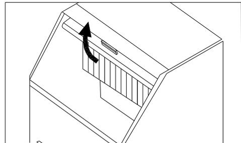
2. Take out the row of flake covers by snapping one end up and pulling forward.
