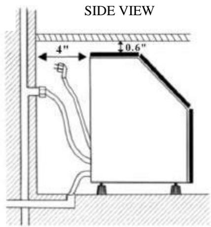
To ensure proper ventilation for your ice maker, the front of the unit must be completely unobstructed. Allow at least 4” (101mm) clearance at rear, and 0.6” (15mm) at top and sides for proper air circulation. The installation should allow the ice maker to be pulled forward for servicing if necessary.
