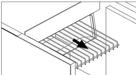
6. Find the sprinkler arm and raise it. Disconnect it from any water tube.
