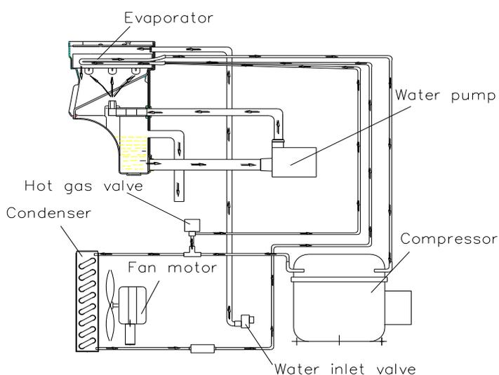
The ice maker begins with a fixed charge of water that is contained in the water bin. As the water is sprayed against the freezing evaporator surface, the portion of water that does not contain mineral impurities will freeze and stick to the ice cube molds. The water containing
