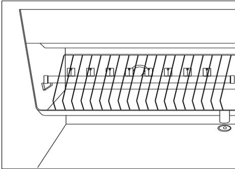
4. Find which water sector is not sprayed well. If the reason is the slideway break the water sector, just adjust the position of slideway to have all the water sectors free forward to the ice mold. If the water sectors are free, but some sector is not sprayed well, using a new teeth-brush clean the gap of the nozzle several times. The water sector will be OK.
