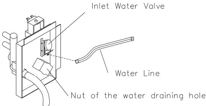
Minerals that are removed from water during the freezing cycle will eventually form a hard scaly deposit in the water system. Cleaning the system regularly helps remove the mineral scale buildup. How often you need to clean the system depends upon how hard your water is. With hard water of 4 to 5 grains/liter, you may need to clean the system as often as every 6 months.
