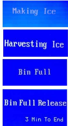
6. When ice cubes are taken out from the ice storage bin, releasing the water curtain, the machine will judge the status for three minutes. During this period, the LCD screen will display the words of "Bin Full Release" and "3 Min To End". "Bin Full Release" flashes until the words "3 Min To End" changes to "0 Min To End". At this time, the ice maker will start to make ice automatically.
