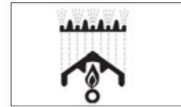
BURNER HEATS RADIANT WHICH RADIATES HEAT TO THE GRATE AND FOOD ITEM.
