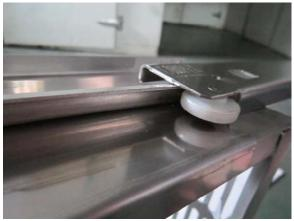
C. Lift drawer and remove from channel.
