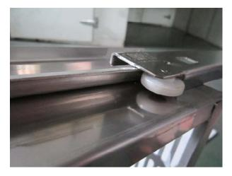
B. make two side tracks of drawer horizontal, lower front rollers into channel.
