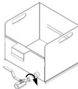
2. Attach valve & nipple (apply thread seal tape)
