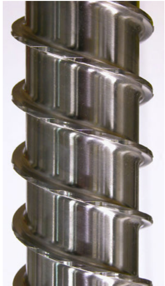
Example of a clean auger
