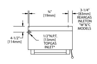
\*Note: TOP GAS INLET pipe extension adds 4" (258mm) to overall height.
