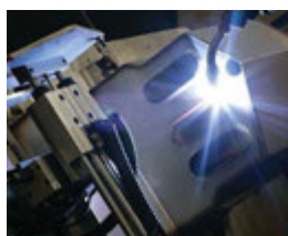
Robotic welding is precise, virtually eliminating leaks.
