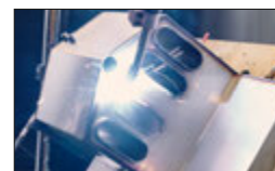
ROBOTIC WELDING IS PRECISE, VIRTUALLY ELIMINATING LEAKS.
