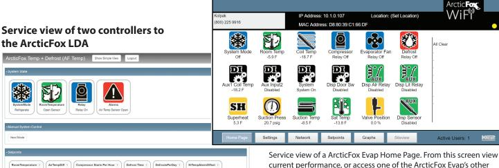
Screen shot of Service view of a ArcticFox Temp. From this screen view current performance, remotely adjust setpoints, name the controller, and manually initiate defrost cycles.
