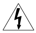
The lightning flash with arrowhead symbol, within an equilateral triangle, is intended to alert the user to the presence of uninsulated "dangerous voltage" within the product's enclosure that may be of sufficient magnitude to constitute a risk of
