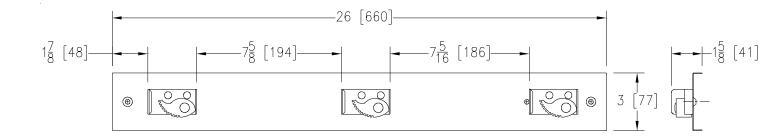
**ENGINEERING SPECIFICATION:** Zurn Light Commercial Z1996-MH Mop Basin Mop Hanger. 26 [660] Long x 3 [76] Wide, 20-gage type 304 stainless steel with three rubber grips.
