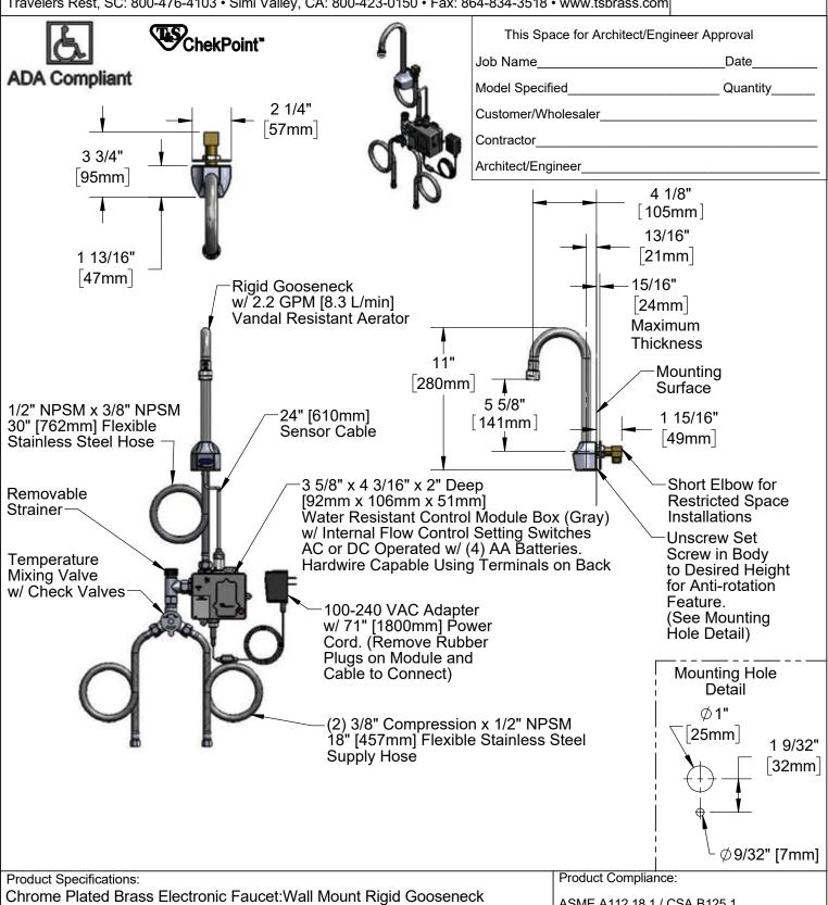
w/ VR Aerator, AC/DC Control Module w/ Internal Flow Control Setting Switches, Temperature Control Mixing Valve w/ Check Valves, 18" Hot & Cold Supply Stop Flexible Connector Hoses
