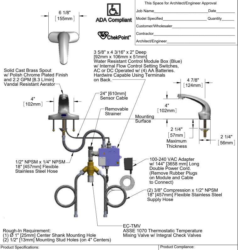
Chrome Plated Brass Electronic Faucet: 4" Centerline Deck Mount Spout w/ VR Aerator, AC/DC Control Module w/ Internal Flow Control Setting Switches, Thermostatic Temperature Control Mixing Valve w/ Integral Check Valves, 18" Hot & Cold Flexible Supply Hoses
