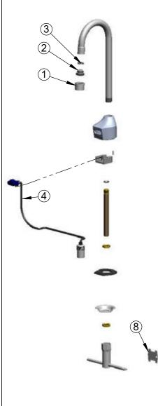
A Maximum of (8) ChekPoint Faucets can be Hardwire Connected and Powered by EC-HARDWIRE ChekPoint Hardwire AC Transformer. (Sold Separately) –
