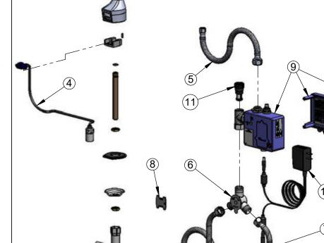
A Maximum of (8) ChekPoint Faucets can be Hardwire Connected and Powered by EC-HARDWIRE ChekPoint Hardwire AC Transformer. (Sold Separately)
