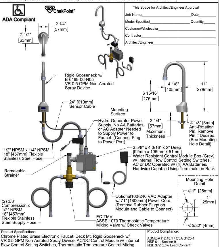
Valve w/ Check Valves, Hydro-Generator, 18" Flexible Stainless Steel Supply
