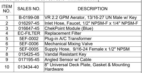
A Maximum of (8) ChekPoint Faucets can be Hardwire Connected and Powered by EC-HARDWIRE ChekPoint Hardwire AC Transformer. (Sold Separately)
