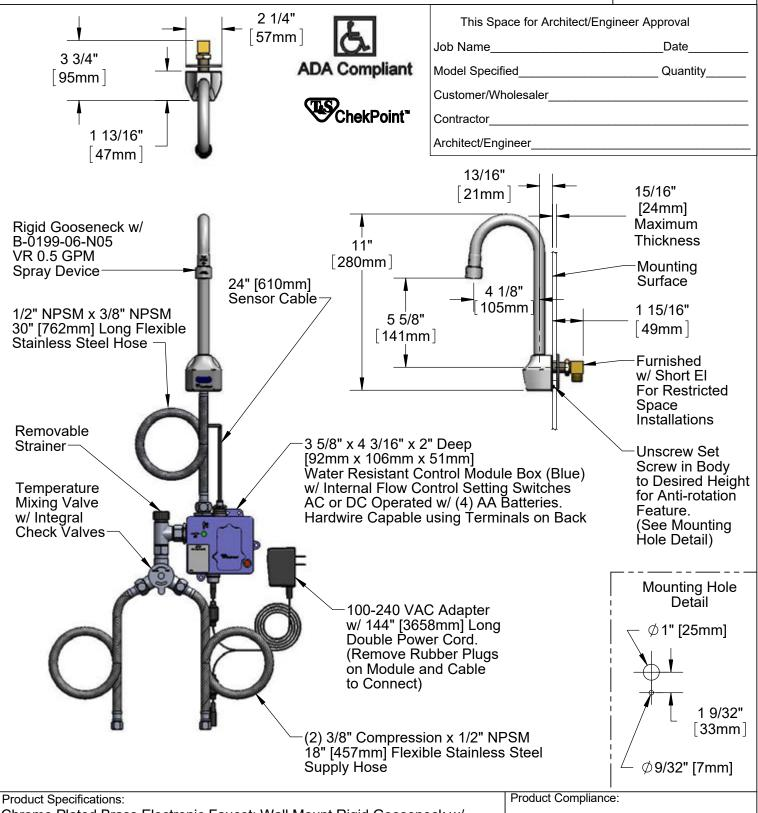
Chrome Plated Brass Electronic Faucet: Wall Mount Rigid Gooseneck w/ VR 0.5 GPM Spray Device, AC/DC Cont. Module w/ Internal Flow Control Setting Switches, Temperature Control Mixing Valve w/ Integral Check Valves & 18" Flexible Connector Supply Hoses
