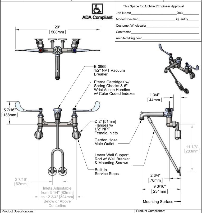
Adjustable Wall Mount Service Sink Faucet, Eterna Cartridges w/ Spring Checks, 6" Wrist Action Handles, Lower Support Rod, 1/2" NPT Adjustable Inlets w/ Supply Stops, Male Garden Hose Outlet, Polished Chrome Finish & 1/2" NPT Vacuum Breaker
