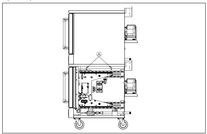
8. Assemble the gas piping shown in the following drawing. Be sure to check all connections for leaks once the oven has been installed.
