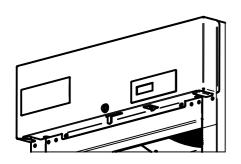
7.- Remove the top head screws, then remove the hinge cap to the right side. Reinstall the top head screws.
