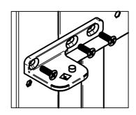
5.- Install the Bottom right hinge in the top left side of the equipment. Then, install the top right hinge in the bottom left side of the equipment.
