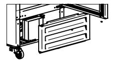
1.— Use the phillips head screwdriver remove the front panel srews, next remove the front panel.
