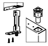
6.—Remove the bottom cartridge and bolt housing from the door, install the cartridge at the top of the door and the bolt housing in the bottom side
