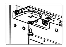
8.—Install the hinges on the left side, but do not tighten the screws. Then install the door and install the cartridge screw. Tighten all screws.
