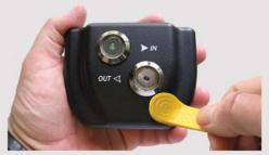
The battery-powered clock can be kept in a truck, a briefcase or a pocket. Employees clock in and out with a *tap* of their iButton.
