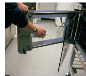
2. Clean back of outer door glass & front of inner door glass.*
