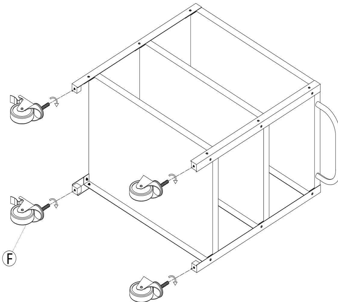
Install the four casters F on the legs and tighten.
