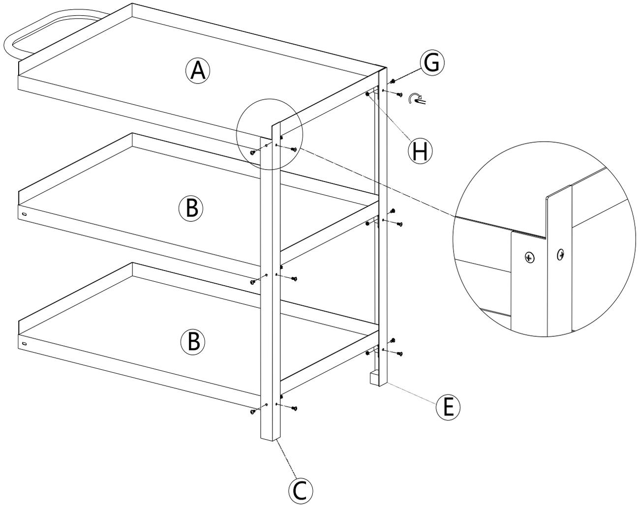
Assemble A, B, C and E together and tighten with hardware G and H.
