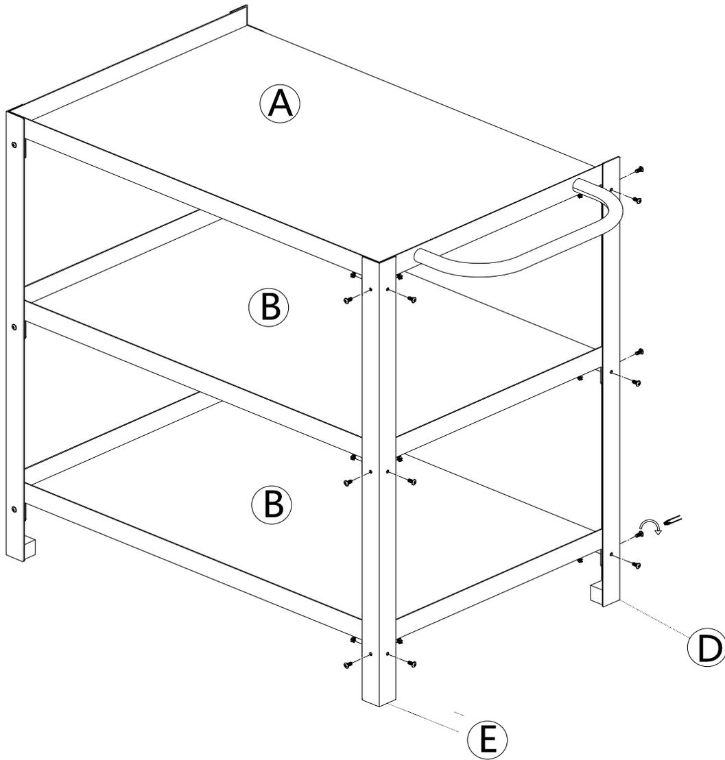
Assemble A, B, D and E together and tighten with hardware G and H.
