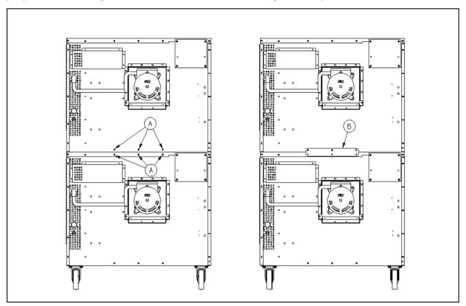
8. Insert two bolts (items "A" in the following diagram) up through the top of the lower oven and screw them into the threaded holes in the bottom of the top oven. Tighten these bolts and the screws that you did not tightened in the previous step.
