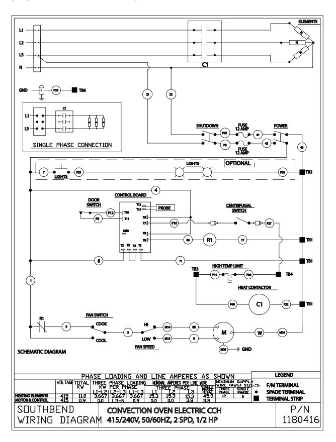
Wiring Diagram for 380/220 Volt Models with Cycle/Cook & Hold Controls
