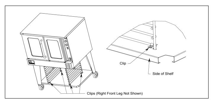
6. Secure the top of the pan-stop to the bottom of the oven with a screw, and tighten the screw holding the pan-stop to the shelf.
