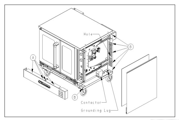
6. Lift the top oven and position it on top of the lower oven, as shown in the drawing below.
