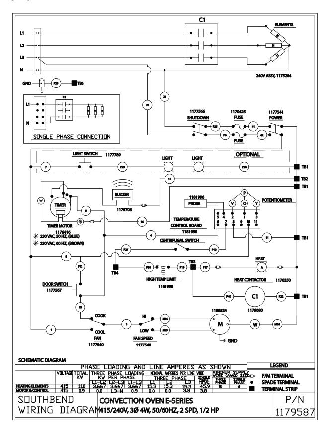
Wiring Diagram for 380/220 Volt Models with Standard Controls
