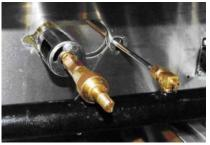
Replace the orifice fittings into the valve.
