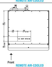
Liquid Ref. Line Electrical Supply 7/8" Dia.Opening **Brazed Line Sets** Suction Ref. Line (Sold Separately) 25' HS-0250 35' HS-0251 55' HS-0252 Voltage supply for the KMS Ice Maker is supplied from the SRK Remote Condenser.
