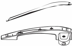
Step 2: Insert the one side of handle cover into the handle pedestal.
