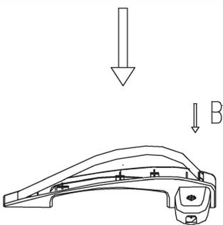
Step 4: Press the cover into the handle pedestal.
