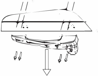
Step 1: Attach the handle on the door with four screws.
