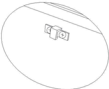
3. Installation of latch hook is finished.
