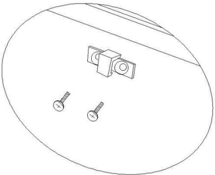
2. Attach the latch hook by lining it up with the holes and attaching it with two screws.
