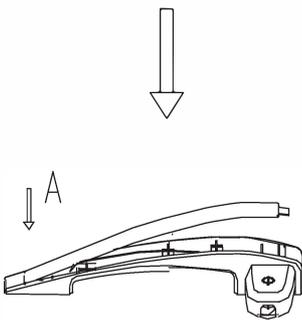
Step 3: Insert the other side of handle cover into the handle pedestal.
