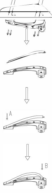
Step 1: Attach the handle on the door with four screws.
